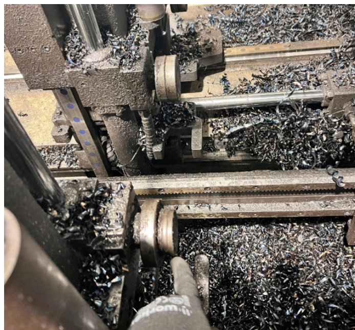
Figure 5B: Machine with cleaning issue
