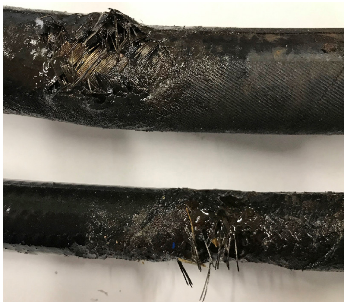
Figure 4B: Damage in hydraulic hose
